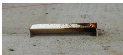
Fig.2. The partial melting effect in the contact area between powder and ammonium nitrate tested
