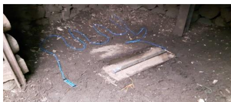
Fig.6 Complete assembly for performing the transition test from deflagration to detonation
