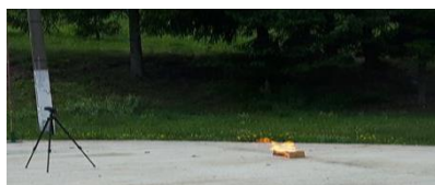
Fig.4 Flame with a tendency to maintain that led to burning a significant part of ANFO
