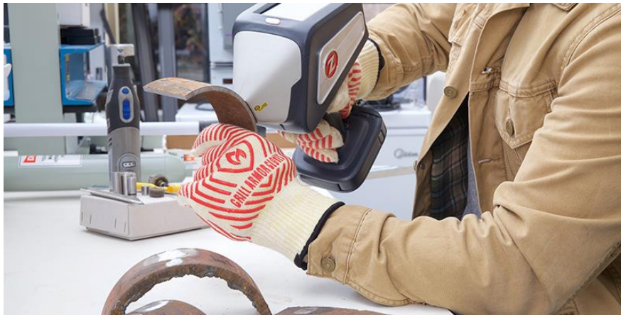
Fig. 5 Sample analysis using the portable laser wave spectrometer Z
