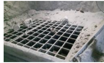
Fig. 9. Rolling collector equipped with grill, mesh size 0.40 X 0.40 m
