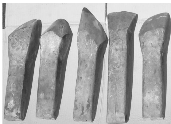
Fig. 3. Variation of the specific wear of the shearer tools depending on rocks abrasion
