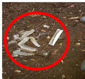
Fig. 10 Test result consisting of the detonation of the test substance highlighted by the destruction of the steel pipe
