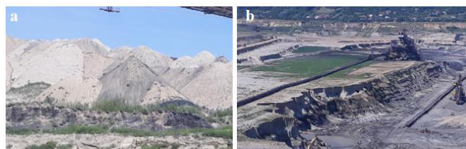
Fig. 4. Inclination of the slopes of the quarry and inner dump during the exploitation period; (a) Inner dump; (b) Quarry
