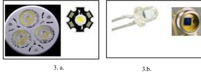
Fig. 3. LEDs (3.a.) and PDs (3.b.) used in our prototypes
