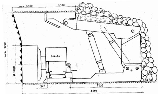
Fig. 3. Cross section of a longwall equipped with sublevel caving shields type VHP742/1 and ESA-60L shearer
