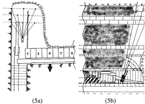
Fig. 5. Crossing of the longwall and the transportation drift (5a) and the vertical section of coal seams and the blastholes along the drift (5b)
