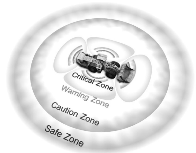
Fig.13. Warning distance in case of collision
