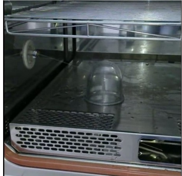
Fig. 4 Spraying the light disperser inside the climatic chamber
