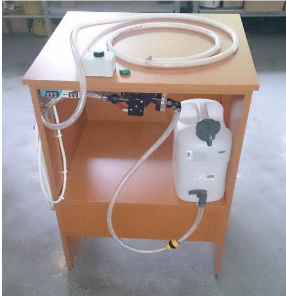
Fig. 3 Test rig for performing the thermal shock test
