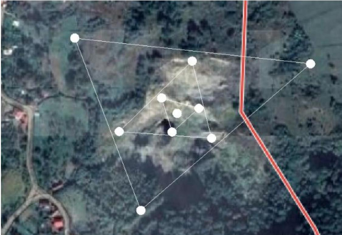
*Fig. 1. Planned positioning of ground control points – year 2021*
