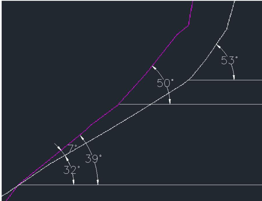
*Fig. 17. Section 1 Southern Part – Slope Inclination – 2021-2022*
