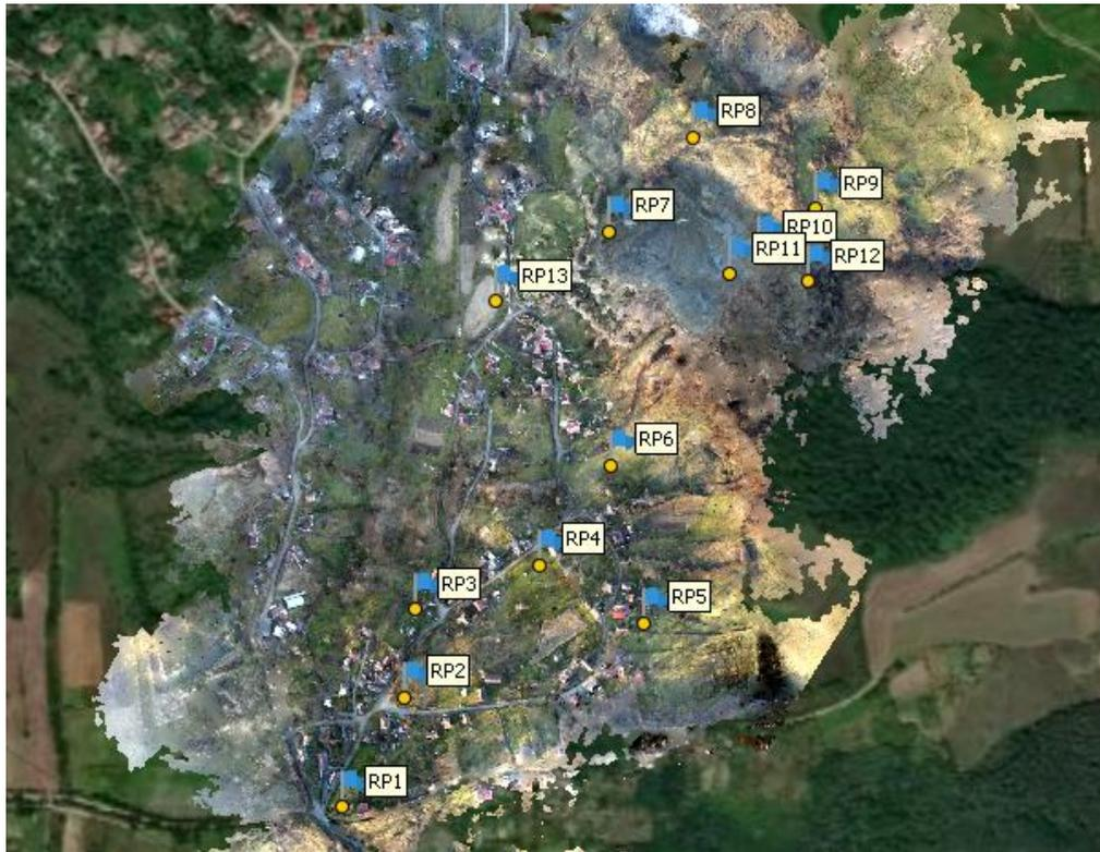
*Fig. 3. Actual positioning of ground control points – 2022*
