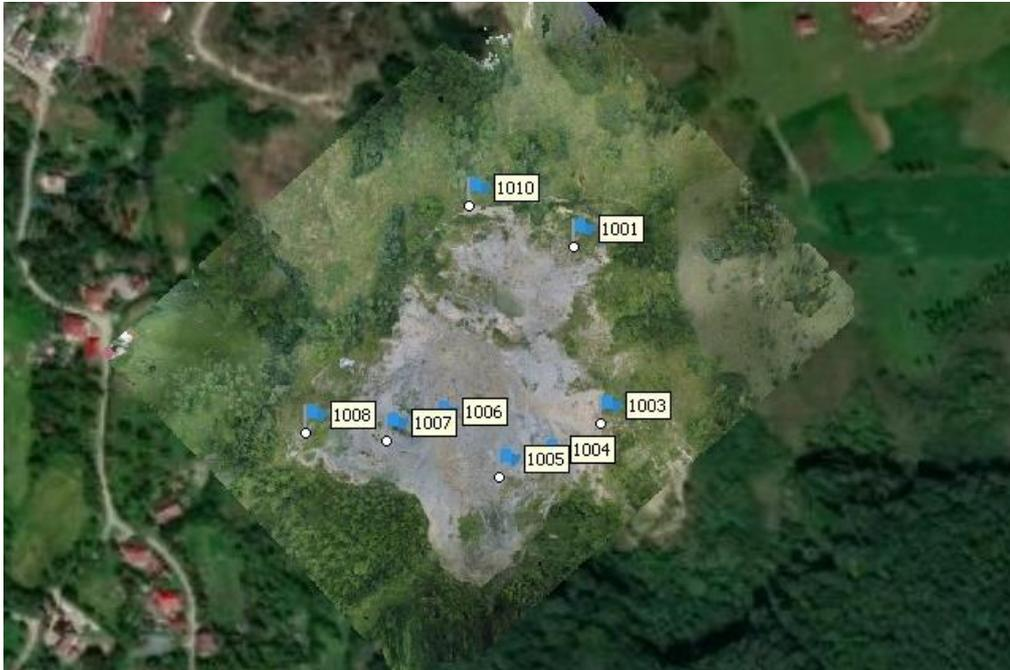
Fig. 10. The central area shows the orthophoto overlaid with the map provided by the software – year 2021
