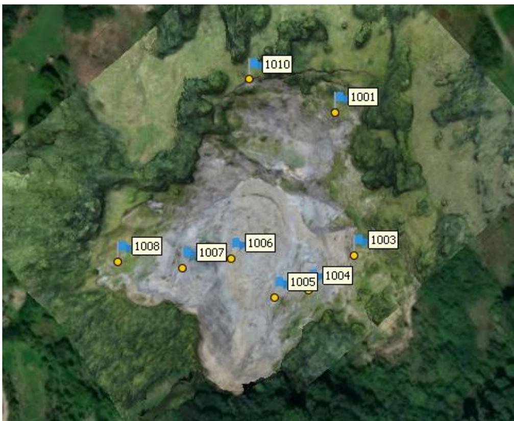
*Fig. 2. Actual positioning of ground control points - 2021*
