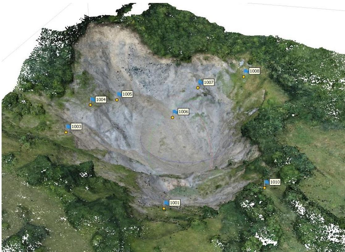
*Fig. 6. Point Cloud and Ground Control Points – 2021*
