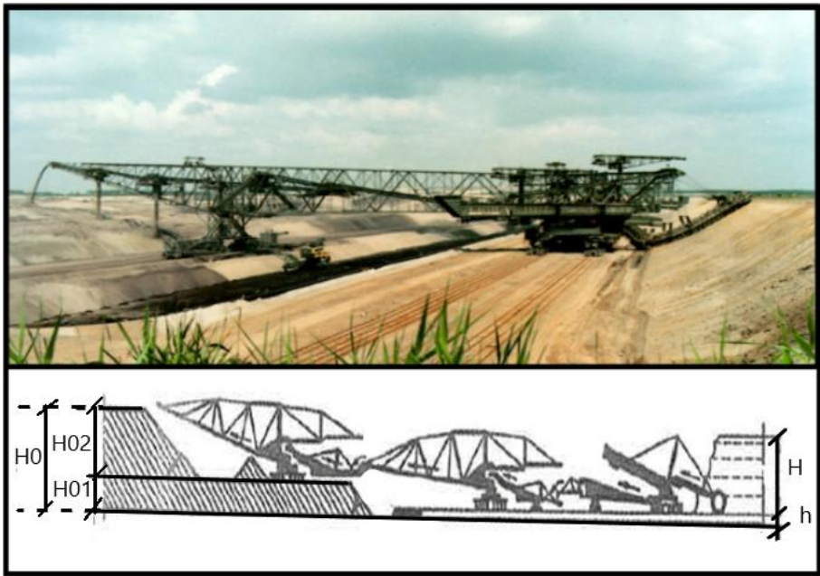
Fig. 18. Mining method with passage of waste rocks to internal dumps, with the use of two ferry bridge whit overhanging arm H – the height of the waste seams, h – the height of the useful seams, H01 – the first step of stored waste H02 – the second step of stored tailings, H0 - the total height of the waste deposit
