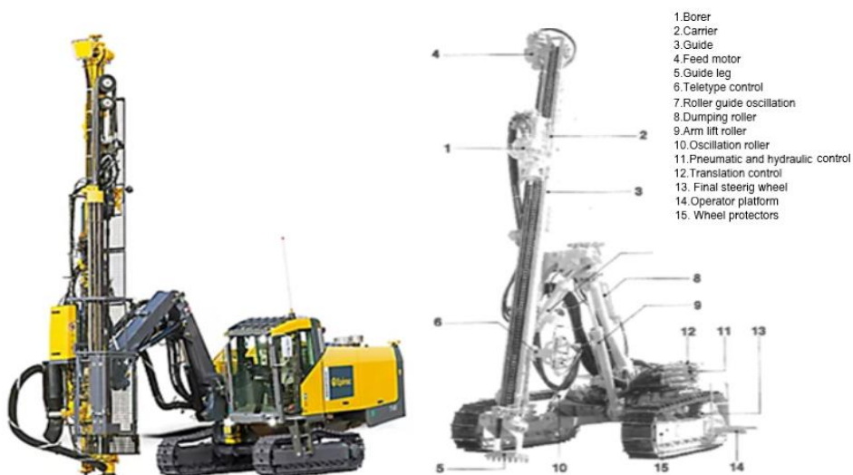
Fig. 5. Drilling rig with the drill outside the bore hole and its components
