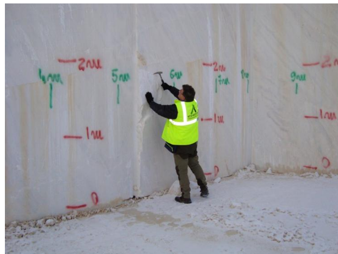
Fig. 3. Field photograph of the Main Wall at Ruschita (white-marble level): horizontal scanline calibration with red 1-metre marks (0 - 9 m) and green vertical control (0 - 2 m). The wall height of 7.5 m and the bench floor are visible. Source: AI-COSTSQO field campaign
