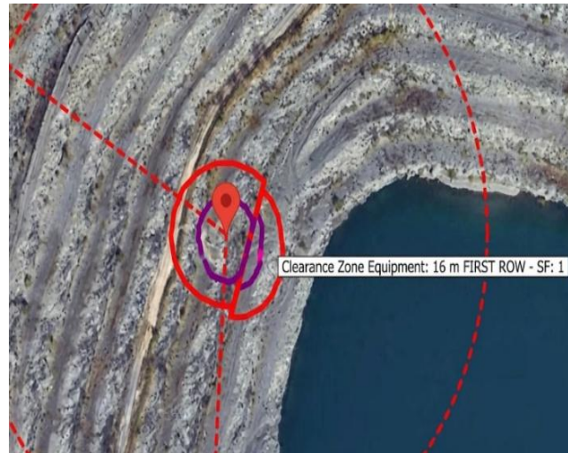
Fig. 4. First blast pattern clearance zones (O-Pitblast screenshot)
