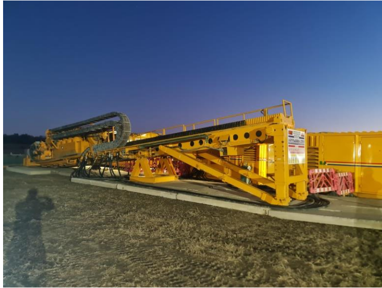
Fig. 1. Directional horizontal drilling unit (HDD rigs)
