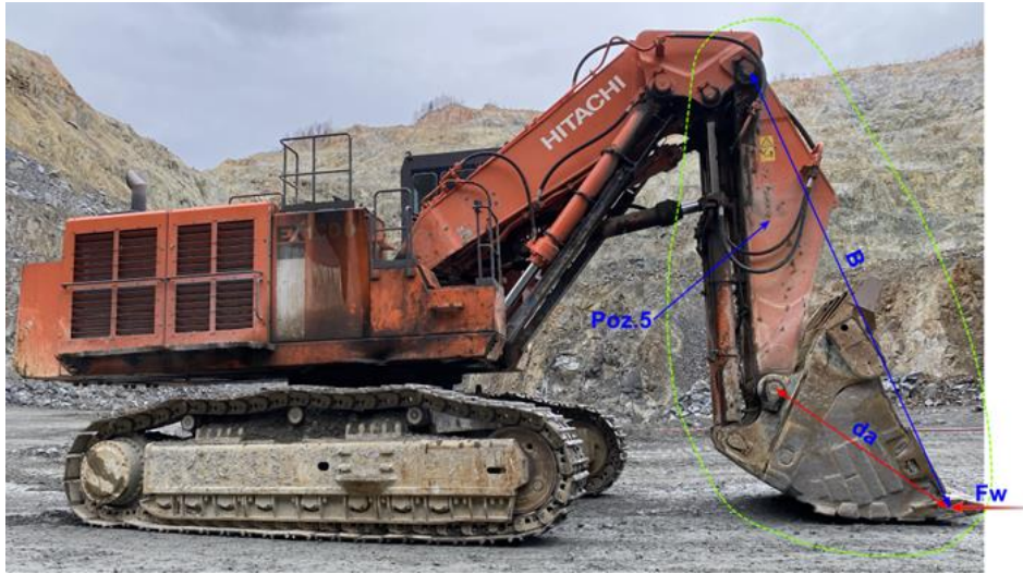
Fig.4. Critical working position of the boom with the action of the force F_w
