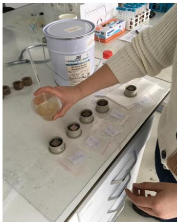
Fig.9. Pouring of the samples into the molds with epoxy resin
