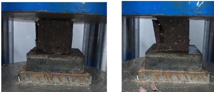
Fig.7. Strength tests of the sample extracted from the mine
