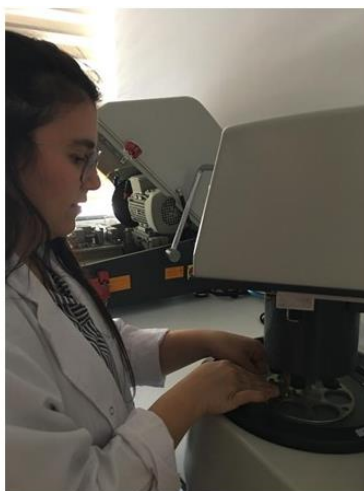
Fig.11. Polishing of samples
