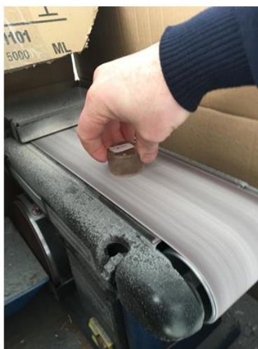
Fig.10. Sanding of the samples molded with epoxy resin
