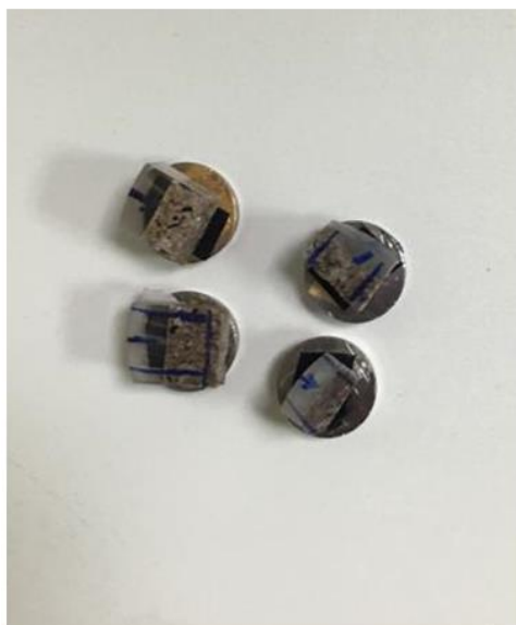
Fig.12. Samples to be gold plated and the gold plating process
