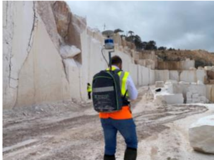
Fig.6. LiDAR scanning using Mobile LiDAR at Onur marble quarry, Turkey
