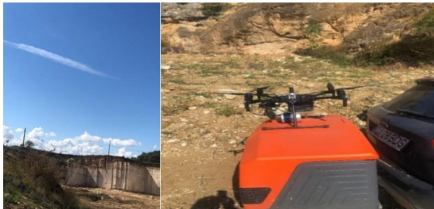
Fig.7. Drone surveying for SfM at travertine quarry - Carpinis, Romania
