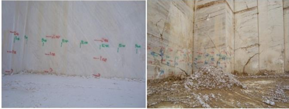
Fig.1. Defining the window sampling at marble and travertine quarries, Romania
