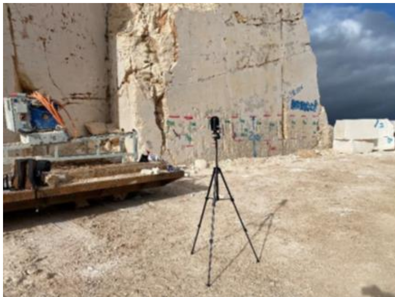
Fig.5. LiDAR scanning using TLS at Onur marble quarry, Turkey
