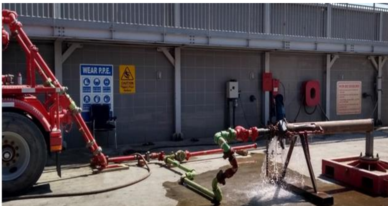
Fig. 3. Casing test stand and high pressure pump
