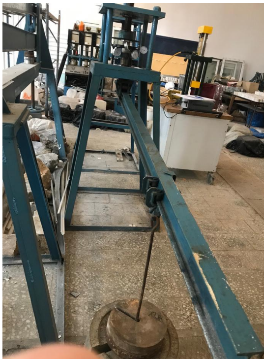
Figure 7. Testing device: Mechanical installation for compression creep tests: a) with a single arm; b) with two arms
