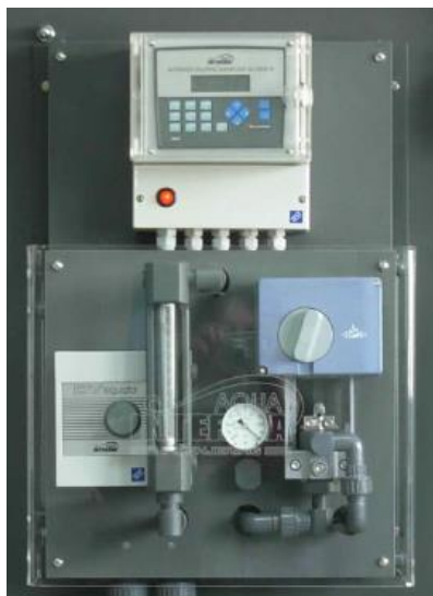
Figure 7. Automatic chlorination unit AS02004/9
