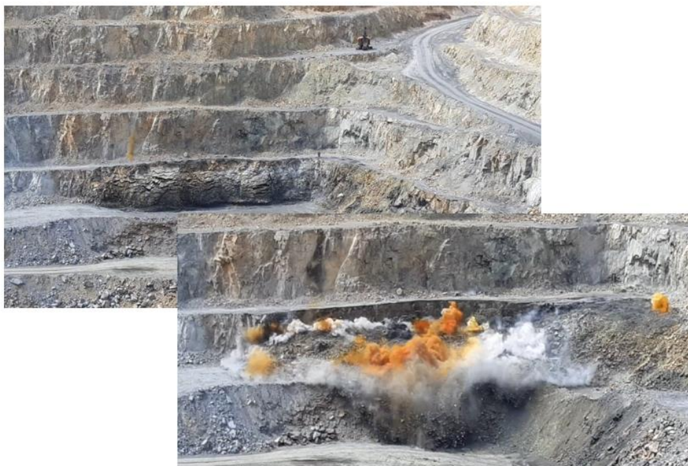
Figure 1. Gas resulting from the shooting – Roşia Poieni
