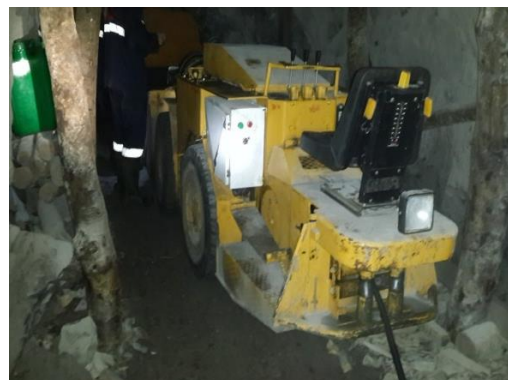
Figure 4. Mini scoop with bucket capacity of 0.5m 3 type ARAMINE
