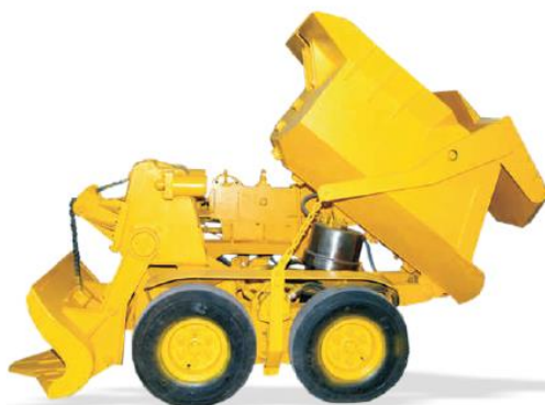
Figure 3. Pneumatic Mucking Machine LHD
