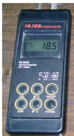
Figure 8. Potable apparatus for the determination of pH, redox potential, temperature, conductivity and dissolved oxygen
