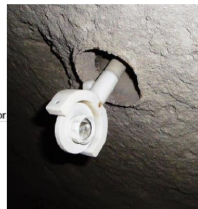
Figure 6. (e): Sketch of the monitoring bolt unit mounted in the shotcrete liner. (f): Bolt and adapter with prism lens mounted in a niche
