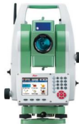
Figure 6. (c): Photograph of the Tachometer, e.g. "Leica, TS 09" of the tunnel underground monitoring
