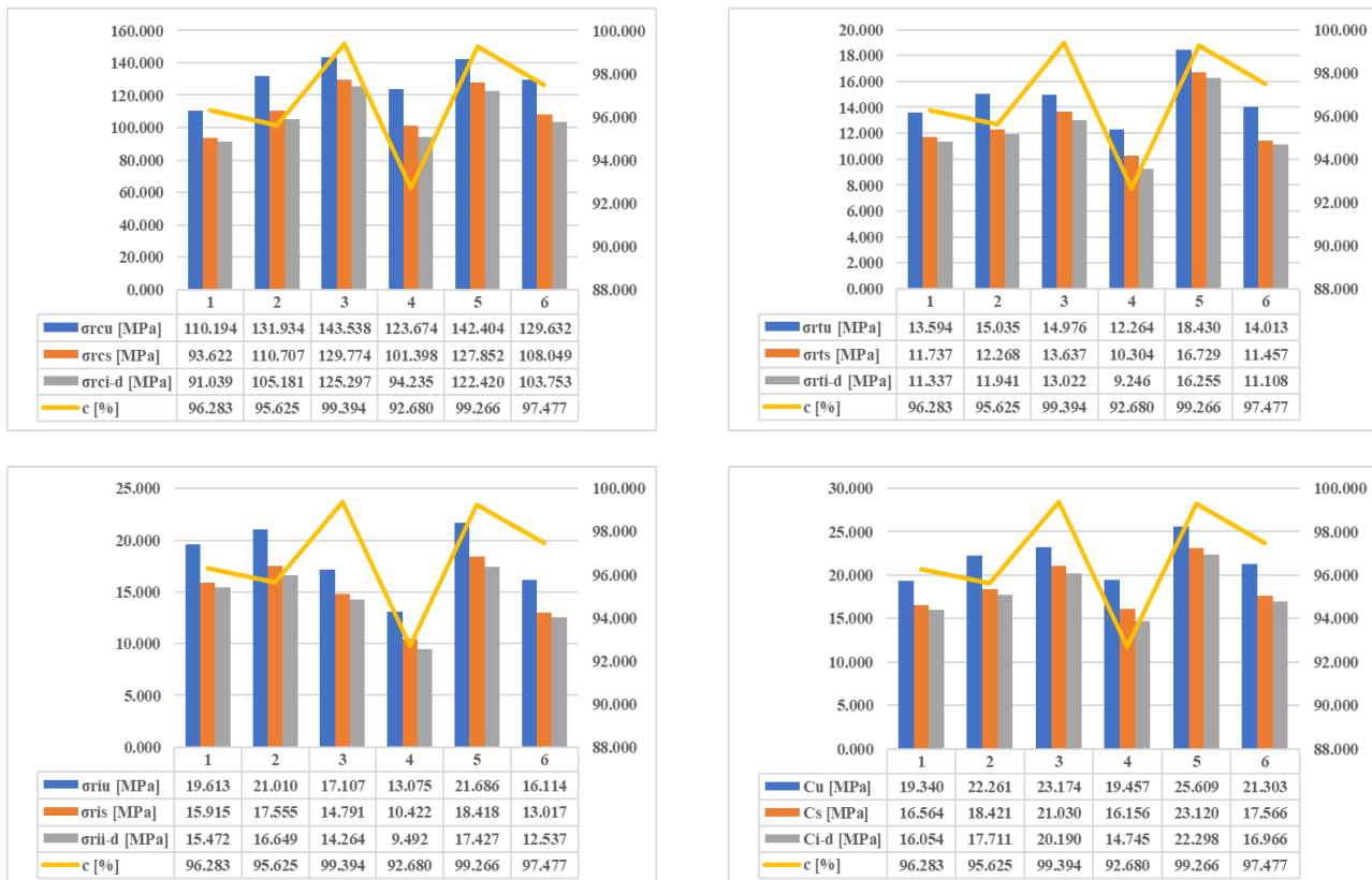
Fig. 11. The influence of compactness on the mechanical characteristics of the tested rocks in dry, saturated state and after freeze-thaw cycles
