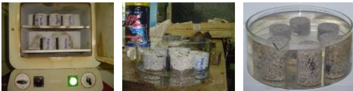
Fig. 4. Determination of water absorption
