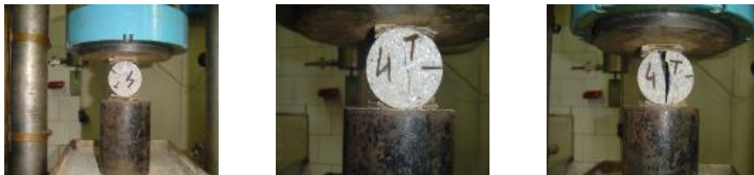
Fig. 7. Determination of tensile strength by splitting (Brazilian method)
