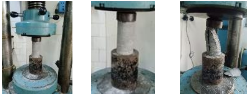
Fig. 5. Determination of uniaxial compressive strength
