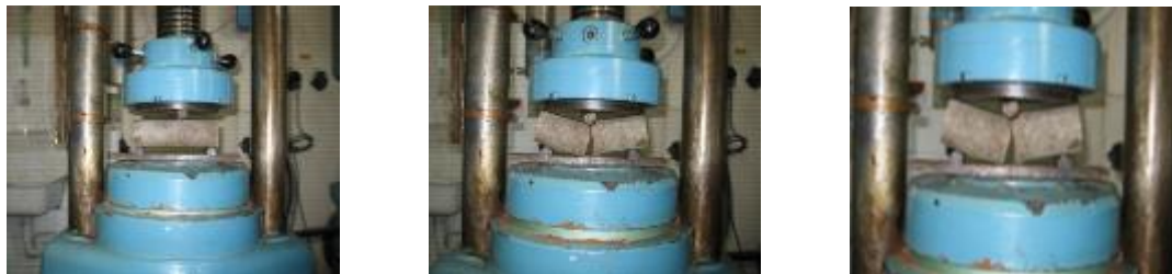
Fig. 6. Determination of bending strength
