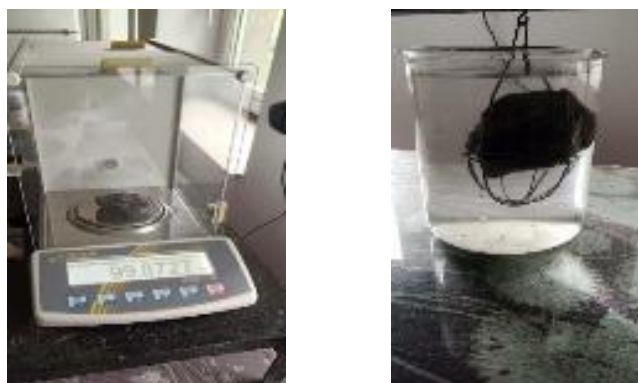
Fig. 3. Determination of bulk density (volumetric) in the laboratory
