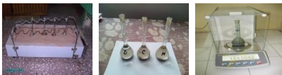
Fig. 2. Determination of real (specific) density in the laboratory
