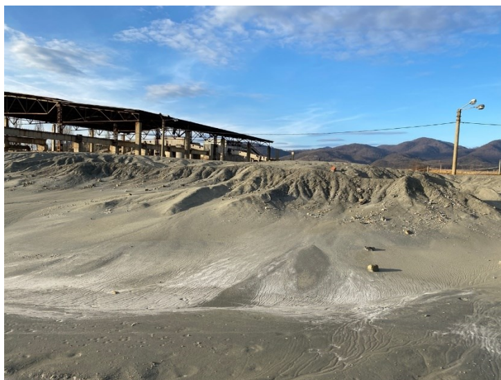
Figure 1 Presence of sulphates formed on the concentrates remaining in the mining perimeter (in dry periods that disappear during precipitation)
