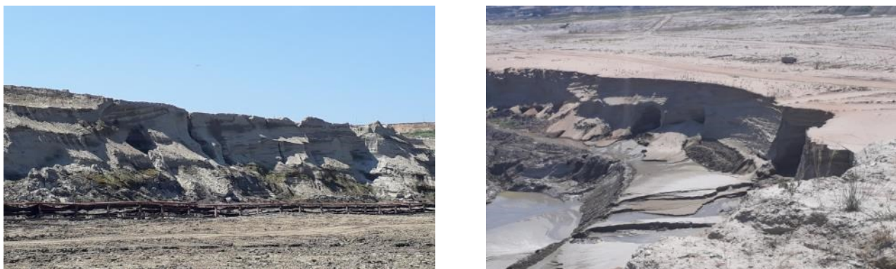
Figure 2. Suffusion zone observed on in-situ slopes
