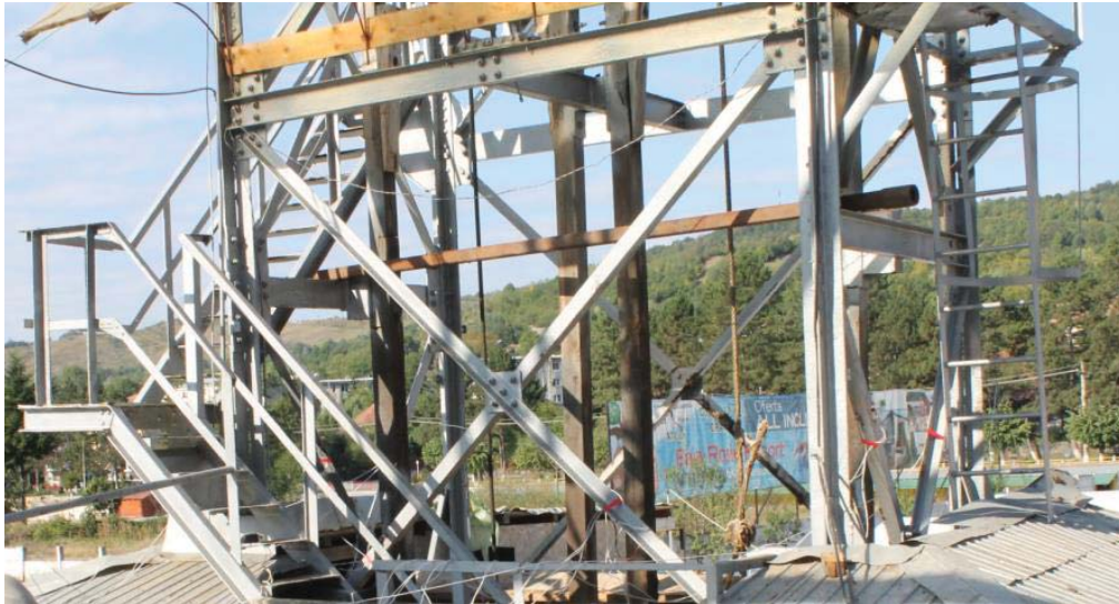
Fig. 16. The location of the strain gauge stamps on the diagonals of the faces' panels
