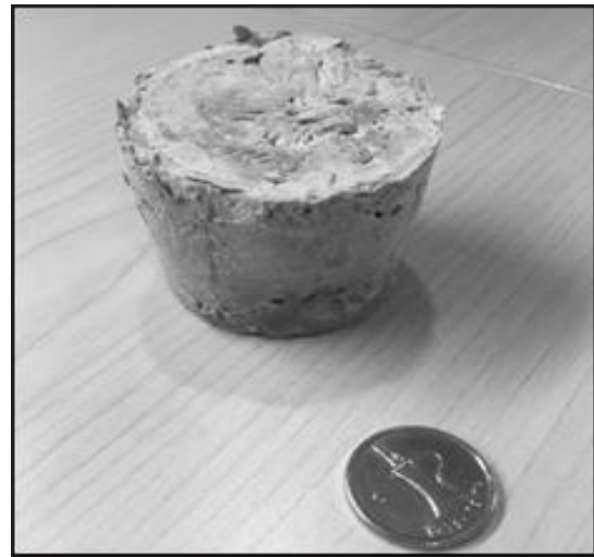
Fig. 2. Diesel based cement Slurry formulation tailored for pumping time
