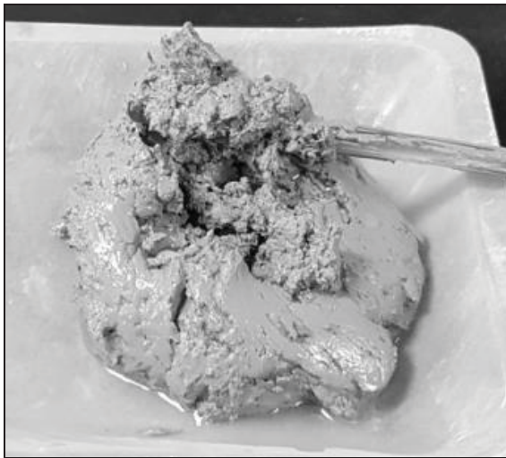
Fig. 2. Diesel based cement Slurry formulation tailored for pumping time
