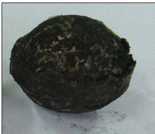
Fig. 5. Briquettes from coal sludge, oil coke, sawdust, \text{Ca}(\text{OH})_2 , lime and molasses
