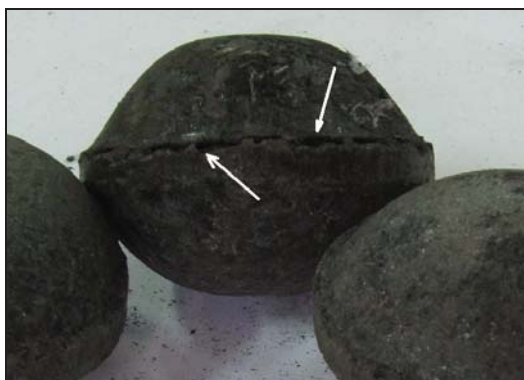
Fig. 6. Cracked briquettes (when recipe 2 was used)
