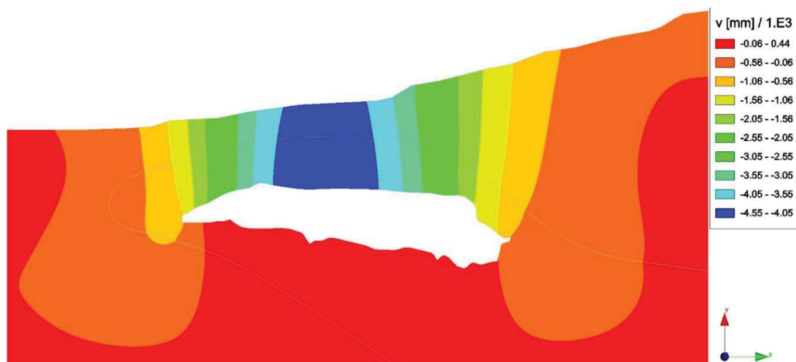
Fig. 7 Vertical displacement of the massive rocks in section 6-6' scalar representation (Option II) – v , in mm
