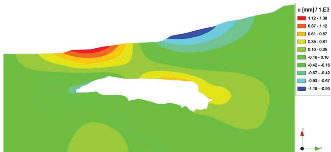
Fig. 9 Horizontal displacements in section 6-6' scalar representation (Option II) – u , in mm
