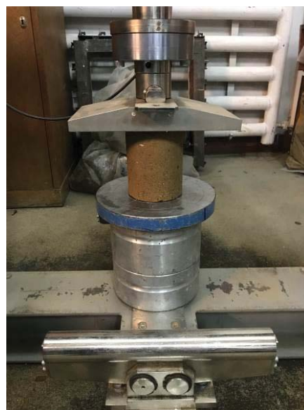
Fig. 7. Determining the compression resistance of a 10cm diameter cylinder
