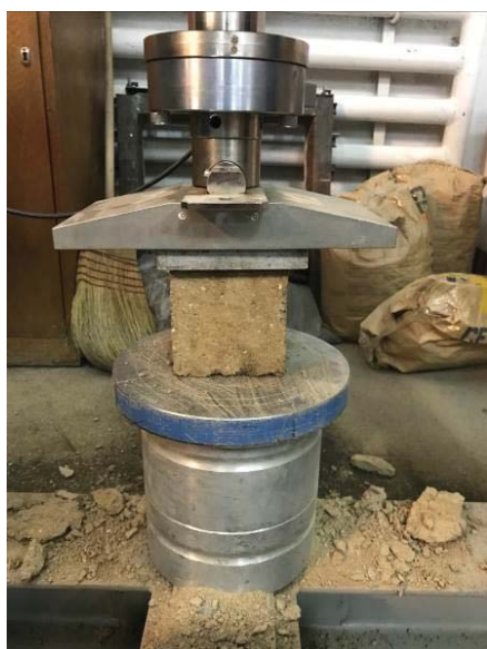
Fig. 6. Determining the compression resistance of a 10x10x10 cm cube
