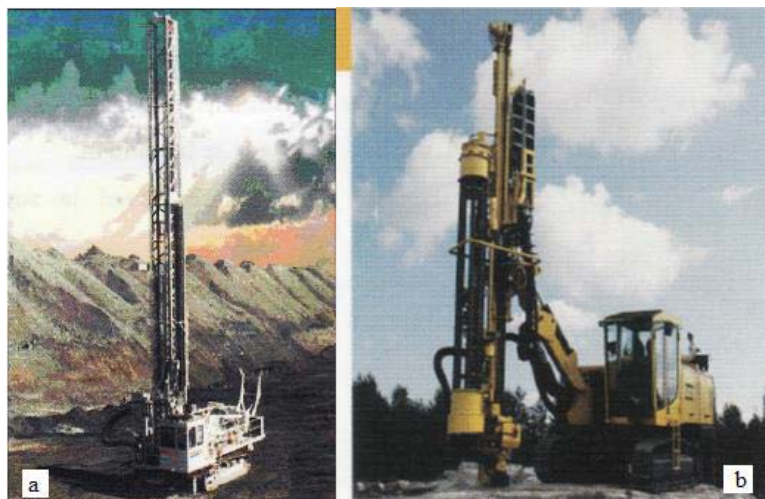
Fig. 4 General view of the drilling equipment in quarries a – Large size rotating equipment for drilling in large quarries b – Rotating – hitting equipment for drilling in useful rocks quarries
