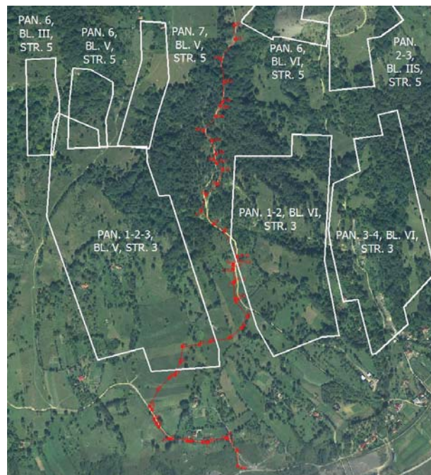
Fig.1 Alignment of subsidence monitoring at Paroșeni Mine
