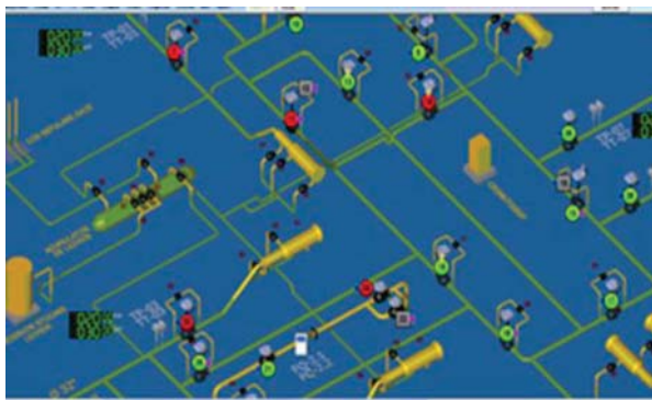
Fig. 4. Synoptic scheme of a storage facility
