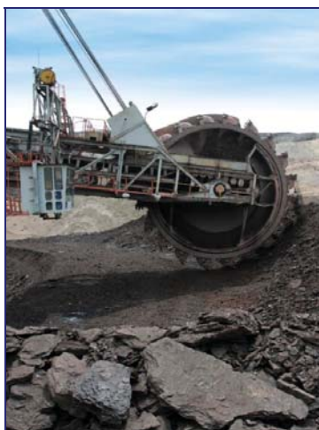
Photo. 4. A bucket wheel excavator with continuous action which extract the useful mineral substance (lignite) in a coal pit from Romania
