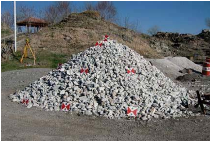
Fig. 4 - Short distance photogrammetry in calculating volumes, in accordance with [5]
