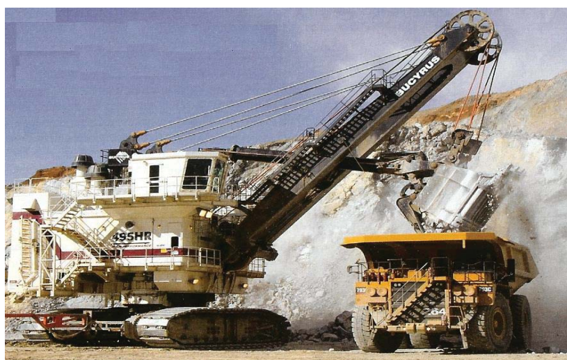
Fig. 9 Excavator loading and vehicle transportation of quarry stuff
