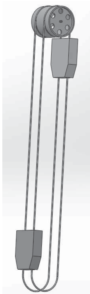
Figure 3 Assembly of statically balanced multi-rope hoisting machinery. The fully loaded transportation container is on the ascending arm
