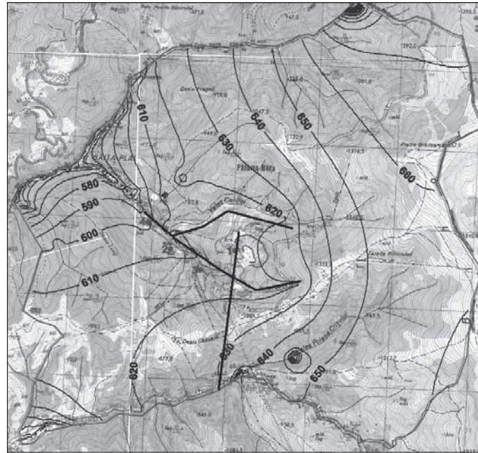
Fig. 3 Piezometric head distribution resulting from a model calibration for K_{matrix} = 10^{-7} m/sec, W_{matrix} = 0.075 mm/day and K_{fracture} = 0.861 m/sec, Paraschivoiu et al., 2014 (map modified from MoND)
