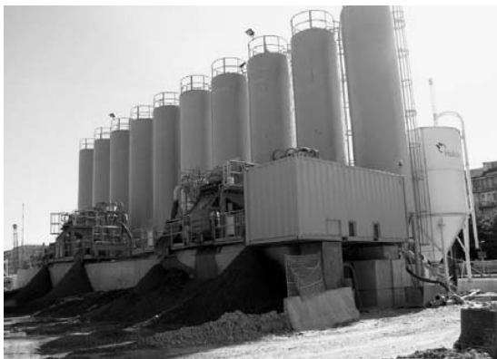
Fig. 4 Compact slurry treatment plant (dewatering, fines separation and partial bentonite recycle) installed for Turin Railway "Passante" works (Oggeri, 2009).
