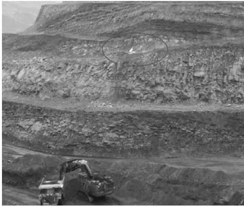
Fig.5. SSR-X radar monitoring a pit footwall from an access ramp
