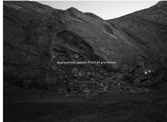
Fig.13 Post failure photograph of June 30, 2006 event showing approximate original location of Prism 41
