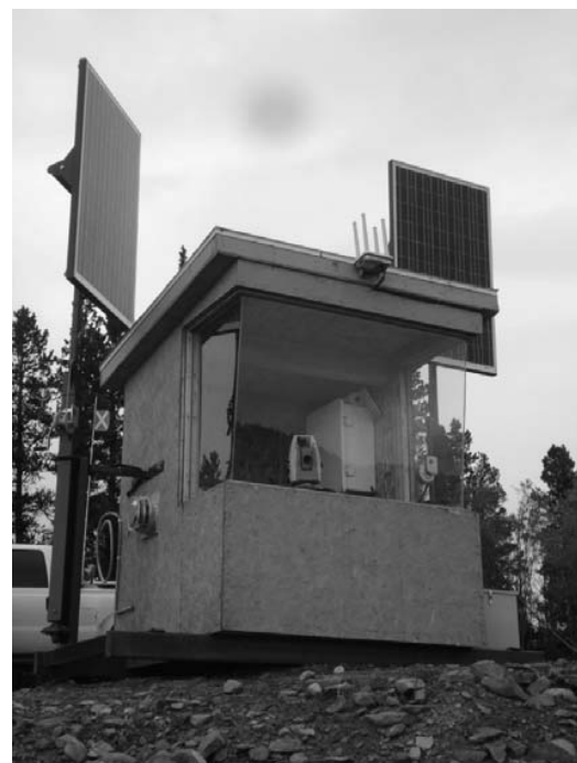
Fig.3. Total station monitoring inside weather protection shelters house
