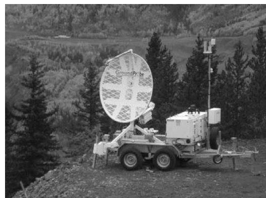
Fig.4. SSR-X radar monitoring system
