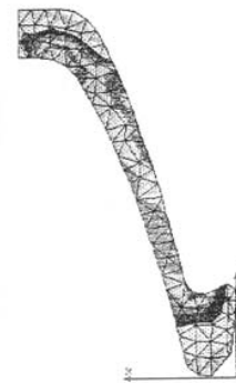
Fig. 8 The distribution of stresses on the height of the bearing section of the laminated profiles: ■- compression maximum residual stress; ■- hog maximum residual stress
