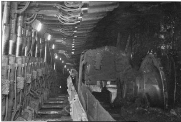
Fig. 6 Perspective of an adit equipped with a mechanized complex 2OKP-70 type and a KŞ-3M shearer
