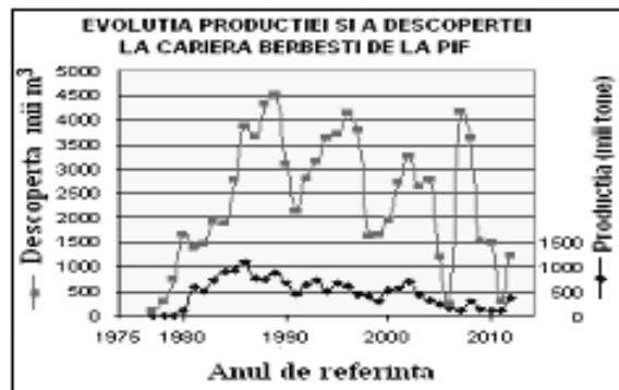
Fig. 10 The stripping and production evolution at Berbești coal pit
