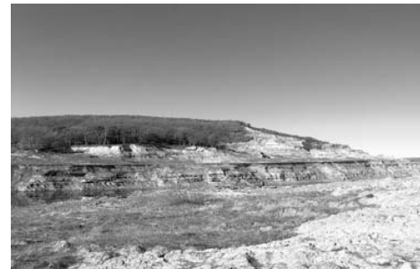
Fig. 6 Sterile dumping in the interior dump by leaning on the final slope of the coal pit
