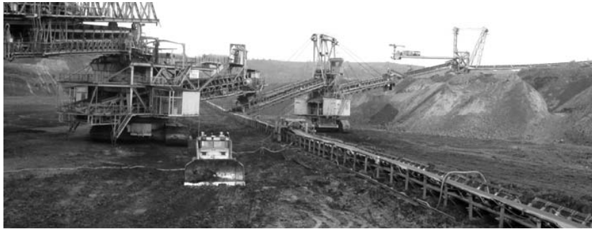
Fig. 9 Sterile transportation on the floor, by a belt truck on tracks, type CBS 1400
