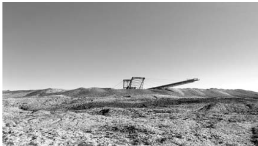
Fig. 6 Sterile dumping in the interior dump by leaning on the final slope of the coal pit
