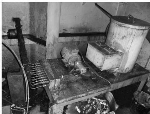
Fig. 2 Modified pipe circuit to the pressure bearing
