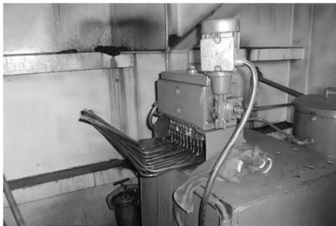
Fig. 1 Initial version of lubrication system to the pressure bearing
