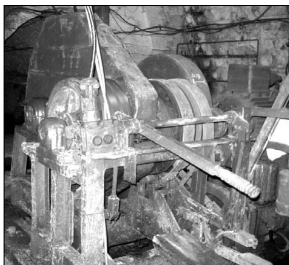
Fig. 2 TPe - 1 x 2000 type electrical mine trolley
