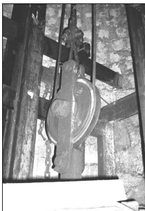
Fig. 5 Mobile pulley to reduce traction force
