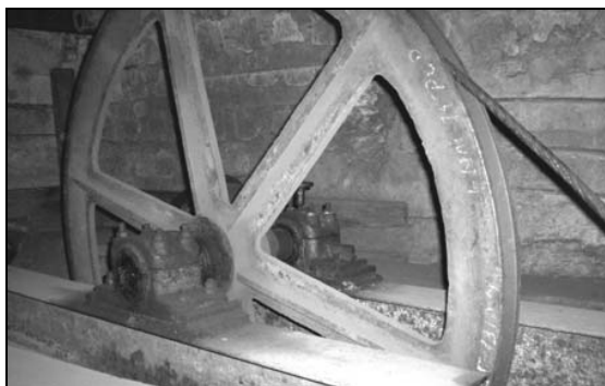
Fig. 4 Deviation winch of the traction cable directing device
