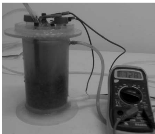
Fig. 2 Microbial fuel cell design: (1) entrance and (6) exit of the feeding solution, (2) zone filled with modified zeolite, (3) anode chamber, (4) cation-exchange membrane, (5) cathode chamber, (7) electricity chain with external consumer, (8) air.
