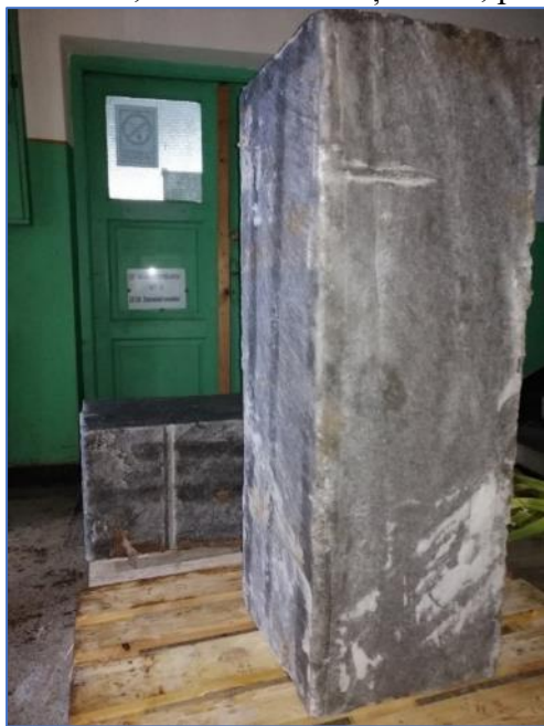
Figura 3. Prisma de sare (400x400x1200mm), Salina Targu Ocna, Bacau
