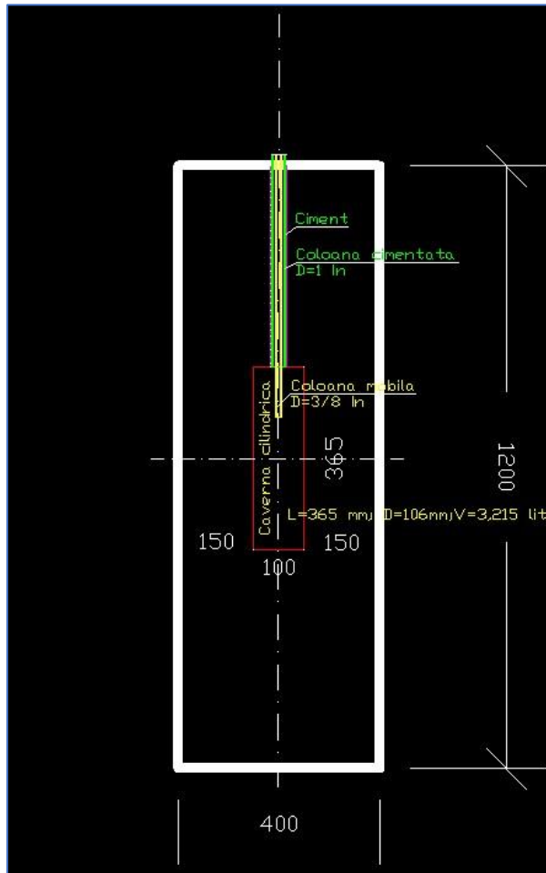
Figure 5. Construction and dimensions of the mini-cavern
