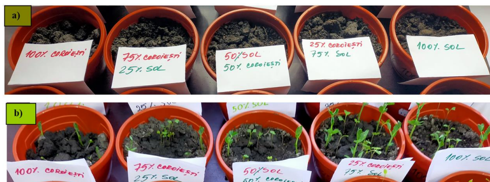
Figure 1. Vegetation pots (Coroiești sterile sludge - fertile soil) according to R1-R5 recipes and plant evolution
