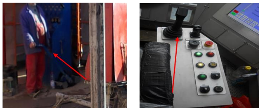
Figure 8. Drill winch brake control lever / "Joystick" control lever
