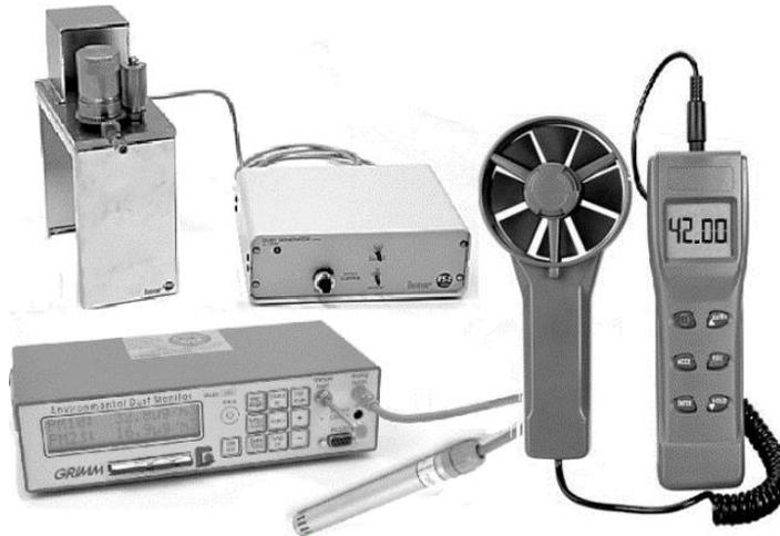
**Fig.1.** Equipment used in the experiment: portable dust monitor (left down); dust generator (left up); portable anemometer (right)
