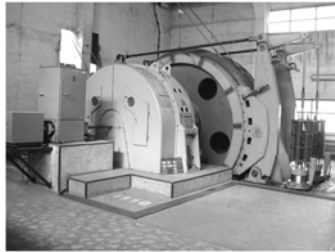
Fig. 2. Two cable drive wheel
