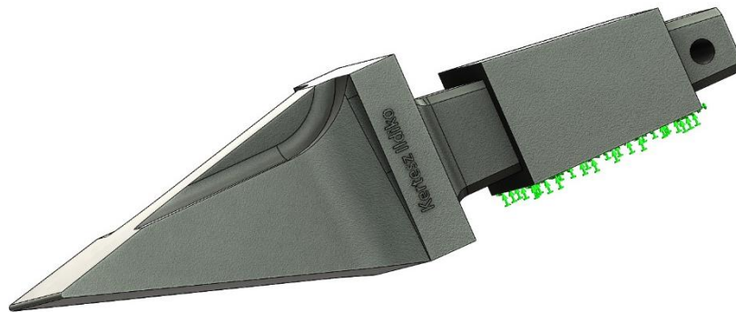
Fig. 8. Fixation conditions of the cutting-tooth
