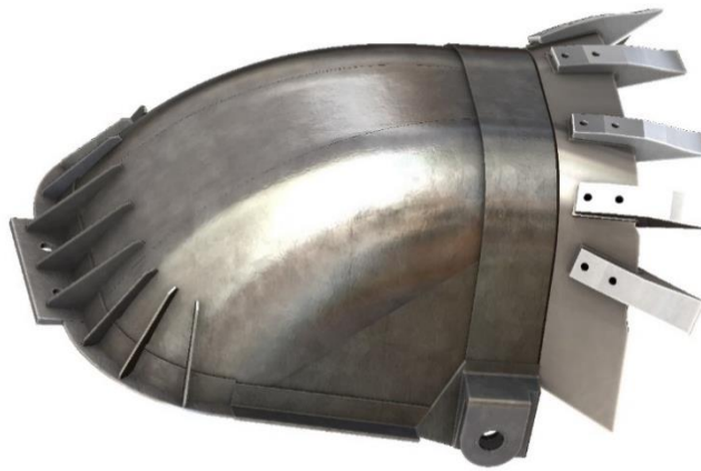
Fig. 4. The bucket with cutting teeth of a BWE
