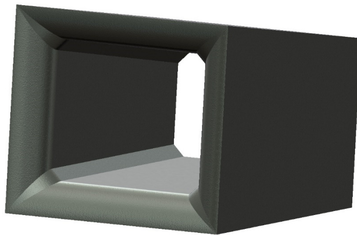
Fig. 8 Proposed holder for fitting the cutting-tooth to the bucket
