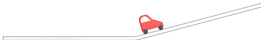
Fig. 6. Position of the vehicle at the initial moment of the dynamic analysis for climbing the inclined section of the driving path
