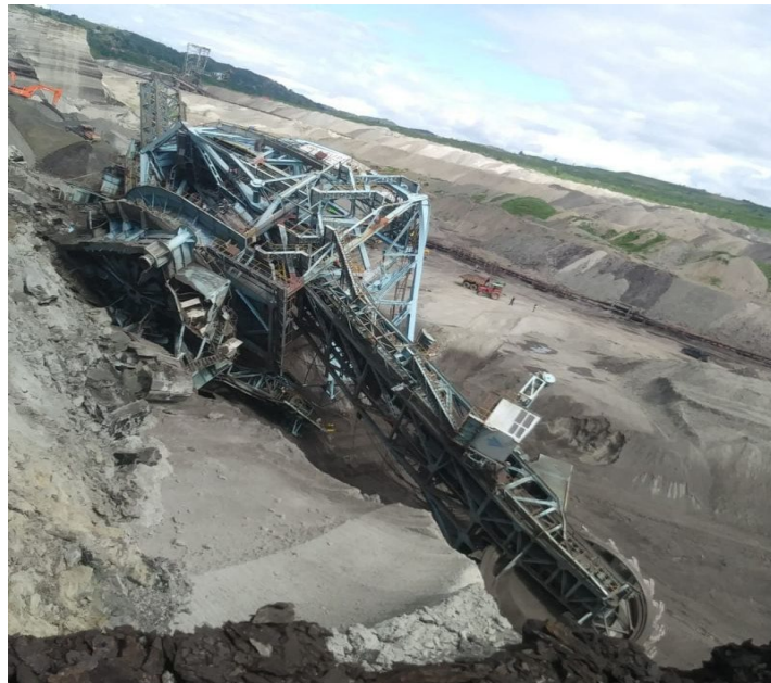
Fig.2. Bucket wheel excavator in Olteania overturned due to landslides caused by heavy rains
